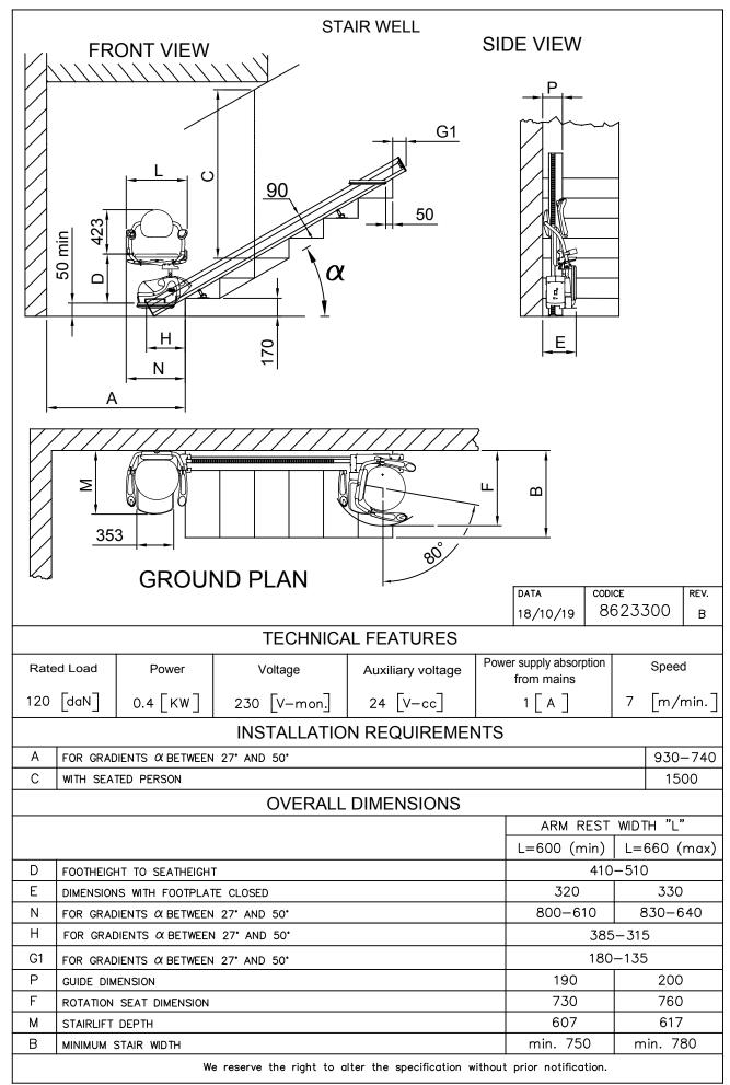
In case of different measurements, compared to "A-B-C", please address to VIMEC technical staff for special applications.
